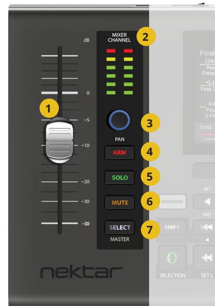
Controlling the selected parameter is a significant, yet easy to use feature. Most mixer, track or channel parameters can be controlled by either the fader or the pan control, including channel volume, levels, MIDI inserts, modulators, instrument and insert plugin parameters. Better still, parameters can be selected for control across tracks. The only exception is instrument parameters which can only be controlled if the instrument is hosted on the selected track.
