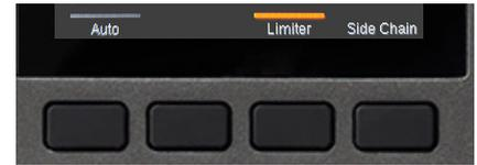
The 4 LED buttons below the 12 pots can also be used for parameter control. If a button is illuminated, it's controlling a parameter. To view the assigned parameter names, press the [DATA/MENU] encoder.
