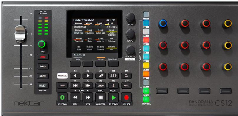
The display shows the parameter assigned to each of the 12 rotary controls. A value indicator is colored to match the rotary control with the parameter name below and value above.
