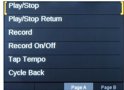
To select an option, press the foot switch and move the [DATA/MENU] encoder. Release the encoder when your selection is made.
